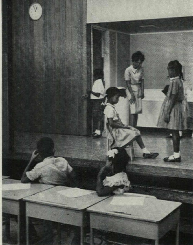
Raised "corridor" end of each classroom (above) serves, among other uses, as a permanent stage. Although classrooms are open-ended, noise has not proved an annoyance, owing largely to acoustic treatment of ceiling and of work alcoves at the corridor end.
