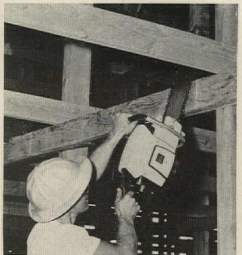
Alloys of aluminum and magnesium account for the engine's lightness. It weighs only 9 pounds by itself, 15 pounds complete with saw. The cost is about \$300.
