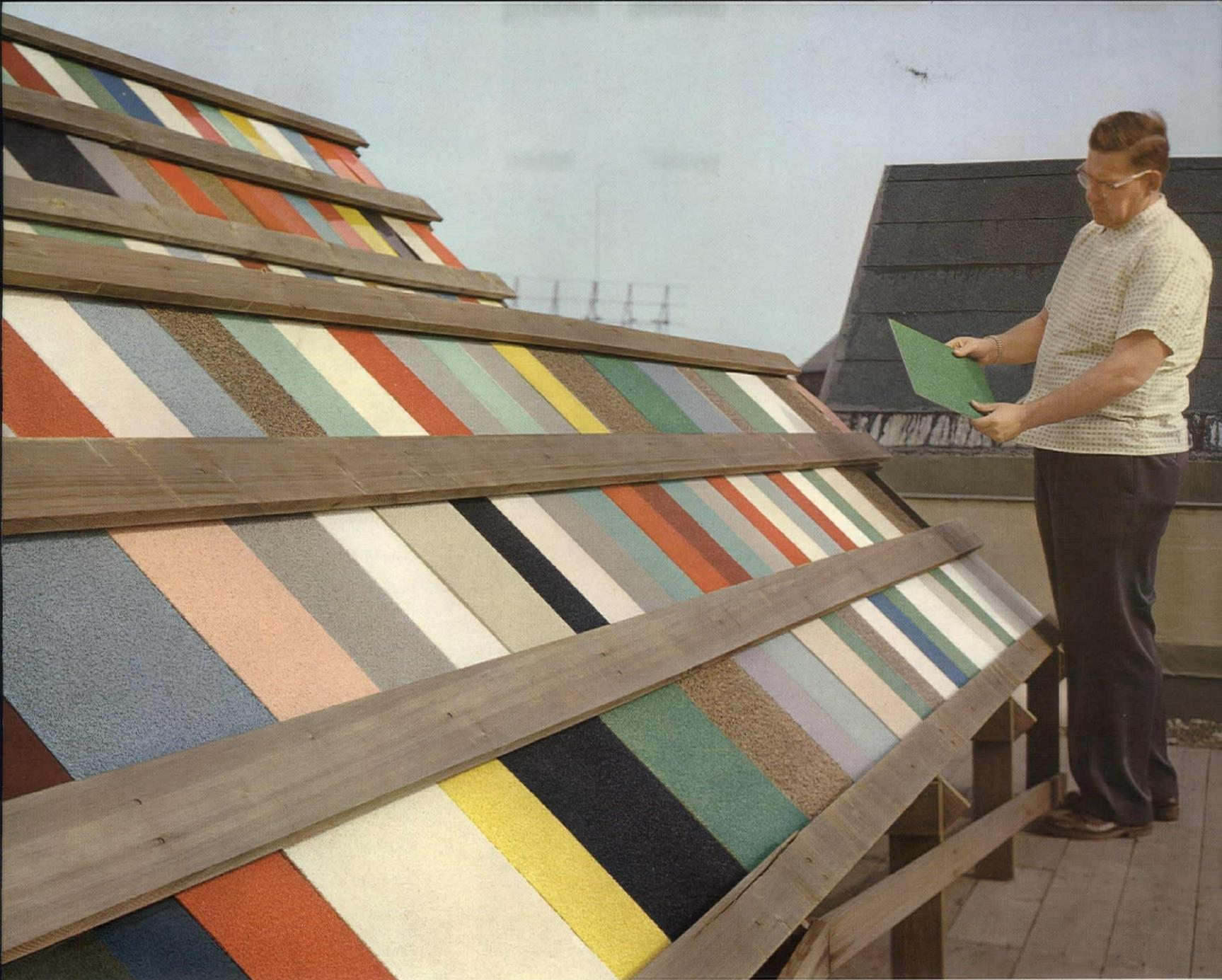
Test fences in Massachusetts and Florida expose Bostik Architectural Coatings to the elements.
