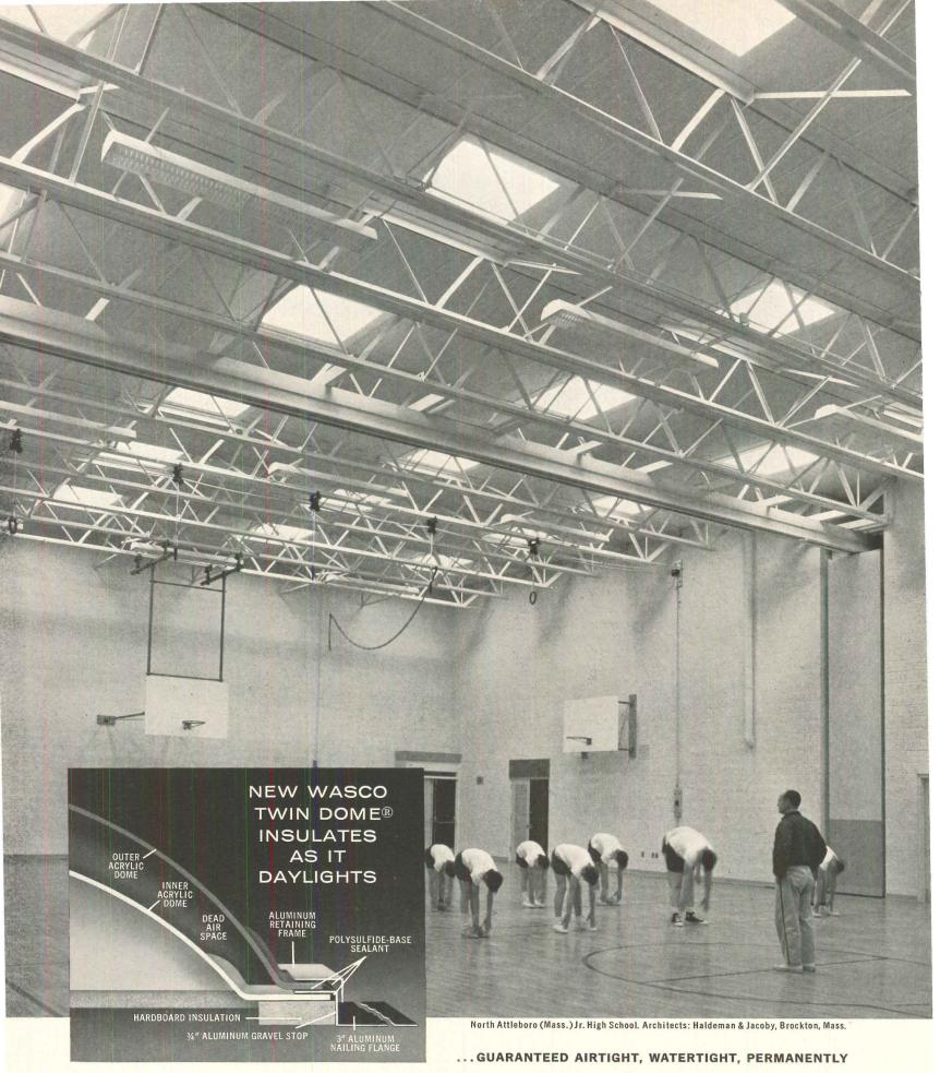
Twenty-eight self-flashing Twin Dome® acrylic skylights illuminate this 5,074 square foot gymnasium without risk of heat gain, heat loss, or condensation. This first totally-proven, permanently-sealed dome-within-dome design is guaranteed watertight and airtight. It maintains a constant 0.57 U-factor. In all, 187 low-silhouette Twin Dome units bring evenly-diffused, glare-
