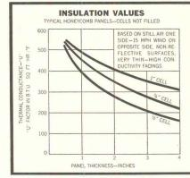
**THERMAL INSULATION.** The sealed-air, cellular construction of UNION HONEYCOMB in panels provides outstanding thermal resistance. Cells can be filled with powdered or granular insulation, or foamable resins, and the resistance increases. Some typical thermal insulation values are shown above.
