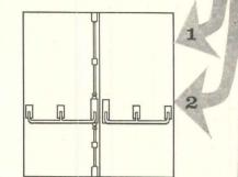
1 New-Pairs. 3 hours U/L "A" label, hollow metal doors to 8° 0° x 8° 0°, single point lock.
