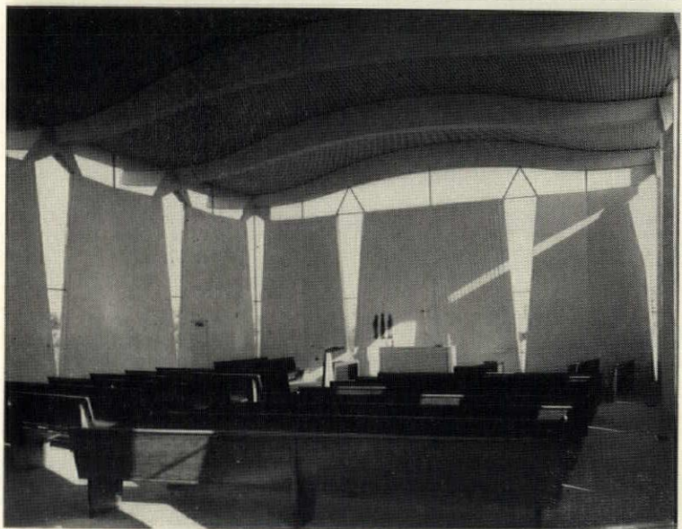
NORTH CAROLINA CHURCH. The faceted glass and concrete walls of the Church of the Holy Infant in Reidsville, N.C. (above) are intended to make the interior "open out into the world around." Precast concrete beams support the wood roof; its deep overhang tilts up to catch more light. A free-standing bell tower contains mechanical equipment. Architects: Schnedl & Schnedl. Contractor: Wade F. Phelts. Cost: $40,000.
