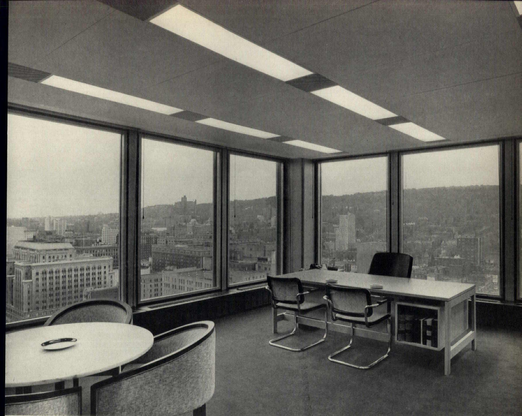
Gray-tinted glass panels, 7 feet high, enclose 14th-floor corner office of Webb & Knapp (Canada) Ltd. Recessed fluorescents are on a 5-foot module.
