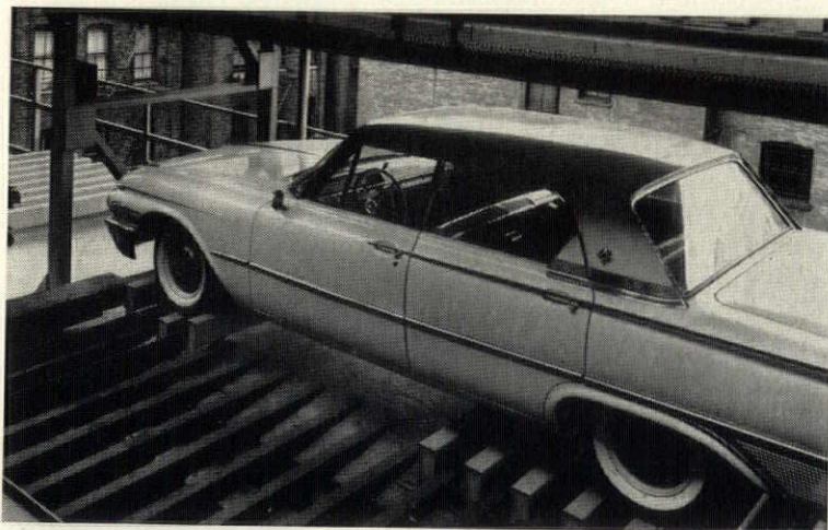
Handling machinery touches cars only at tire treads, minimizing chances of damage. Above, fork-
