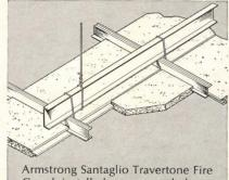
Guard installed on concealed zee suspension system (no intermediate fire protection needed).
