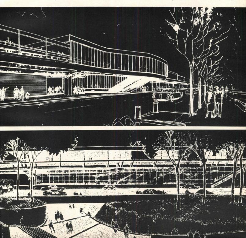
BART was able to squelch an architects' revolt, but it has yet to master its budget problems feet long; a Canopy sheltering the platform, always 280 feet long; a Station Core near the covered portion of the platform, which must be in operation at all times while other areas are closed off during slack hours; and service spaces for electrical and mechanical equipment.
