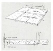
We rabbeted all four sides of our new Armstrong Tegular Travertone<sup>TM</sup> ceiling panels. When you lay them in, they extend 11/32'' below the exposed grid, creating a bold, dimensional effect that's enhanced by the fissured Travertone design. And note how the dimensional effect can be attractively accentuated by painting the grid, as seen above.
