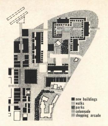
The platform level (above) is given over to the pedestrian; broken lines are pathways through arcades in major buildings. Vehicles have a lower level of their own (below). The section opposite shows the tall, enclosed shopping arcade that will be the main pedestrian "street."
