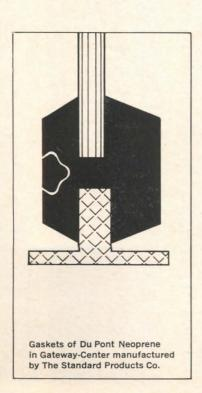
More than 3600 windows and panels in the Gateway-Center Building, Chicago, are sealed with preformed compression gaskets made of Du Pont Neoprene.
