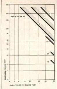
Above, weights of glass recommended by one manufacturer for resistance to sonic boom pressures. Below, the distribution of damage measured in government tests (page 87).
