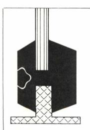
Gaskets of Du Pont Neoprene in Gateway-Center manufactured by The Standard Products Co. More than 3600 windows and panels in the Gateway-Center Building, Chicago, are sealed with preformed compression gaskets made of Du Pont Neoprene.
