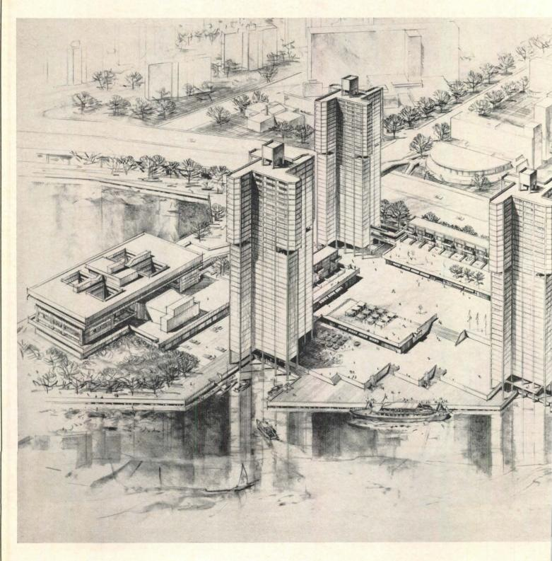
not yet been worked out. It would incorporate multilevel parking decks for about 750 cars, reached from a service road running along the east side of the drive.
