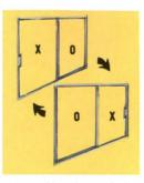
It's **reversible!** The fixed door may be placed left or right... on the same basic frame now or later. Glass requirements may be changed at any time from '/4" glass to insulating glass with only the change of vinyl.
