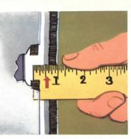
Deeper penetration (9/16 inch) of stile into jamb offers better weather seal. The deep-set jamb maintains its tight seal from top to bottom to compensate for building settlement and less than perfect installation.
