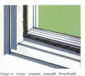
prevents heels from catching in door guides. Threshold cover provides a completely engineered drainage control. Polypile weatherstripping at **both sides of door stiles** and top rail provides positive weather seal for both **inward** and **outward** wind pressures. It's resilient, mildew and rot-proof.
