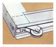
Telescoped corner construction working in conjunction with roller assembly housing creates a strong, rigid, positively positioned corner. Stainless steel rollers with sealed, unitized ball bearings offer full 1/2 inch adjustment.
