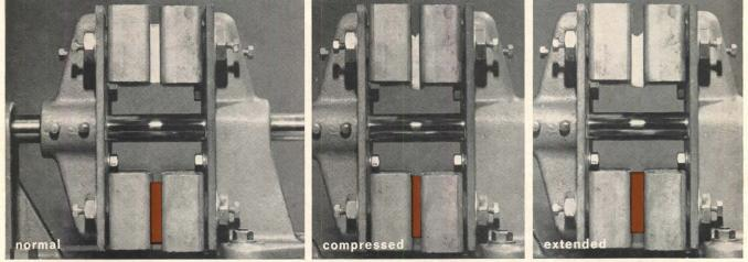
Joint Movement Simulator. Laboratory device permits simultaneous evaluation of sealant compounds. Cycled through compression-extension motion, movement duplicates physical stresses met by installed sealants as dynamic building joints are subjected to natural thermal and structural
