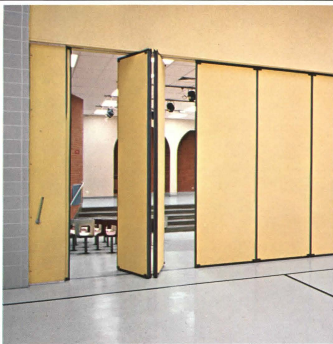
Acousti-Seal 51—for critical sound control requirements—maximum single width: 64'—maximum height: 18'—hanging weight: 7.5 lbs. per square foot of opening—S.T.C. of 51 in 14' x 9' test opening.
