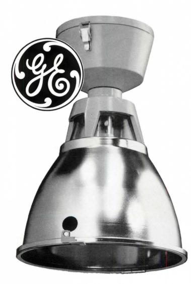
Activated charcoal filter traps airborne contaminants – greatly extends illuminating efficiency. An activated charcoal filter between the lightproducing fixture interior and the dirtproducing plant environment keeps dirt and fumes away from lamp, reflector, and inside door glass. The results: lighting efficiency remains high for prolonged periods; maintenance and cleaning requirements are reduced.
