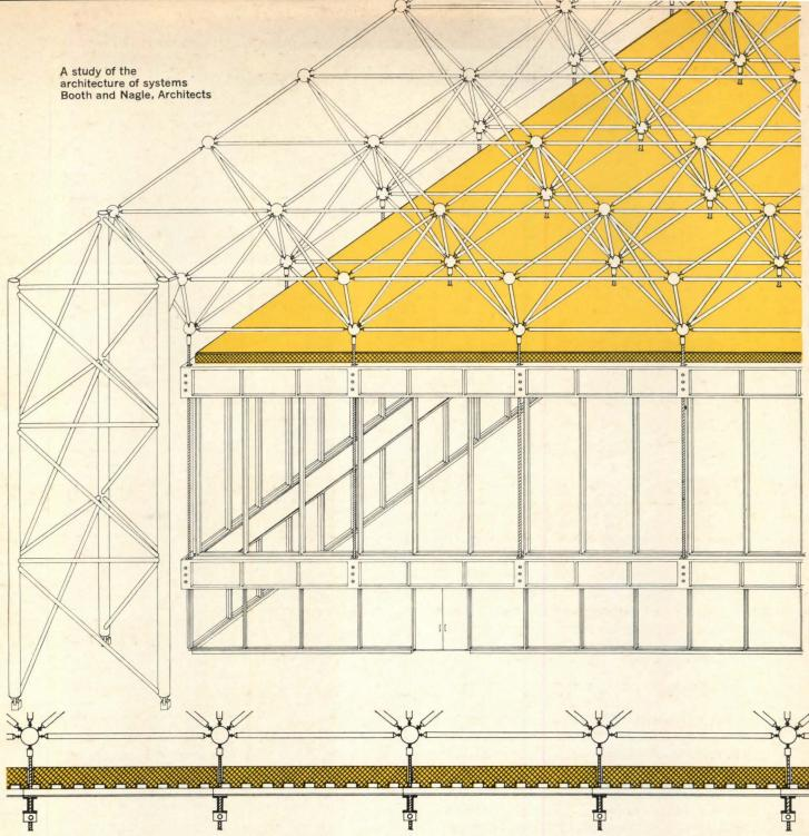
Instead of using structural steel like wood, as is customarily done, this design takes advantage of the tensile strength inherent in the material. A triangular lightweight-steel spaceframe spanning 250 feet is assembled on the ground and raised into position by hoists that are supported by tripods
