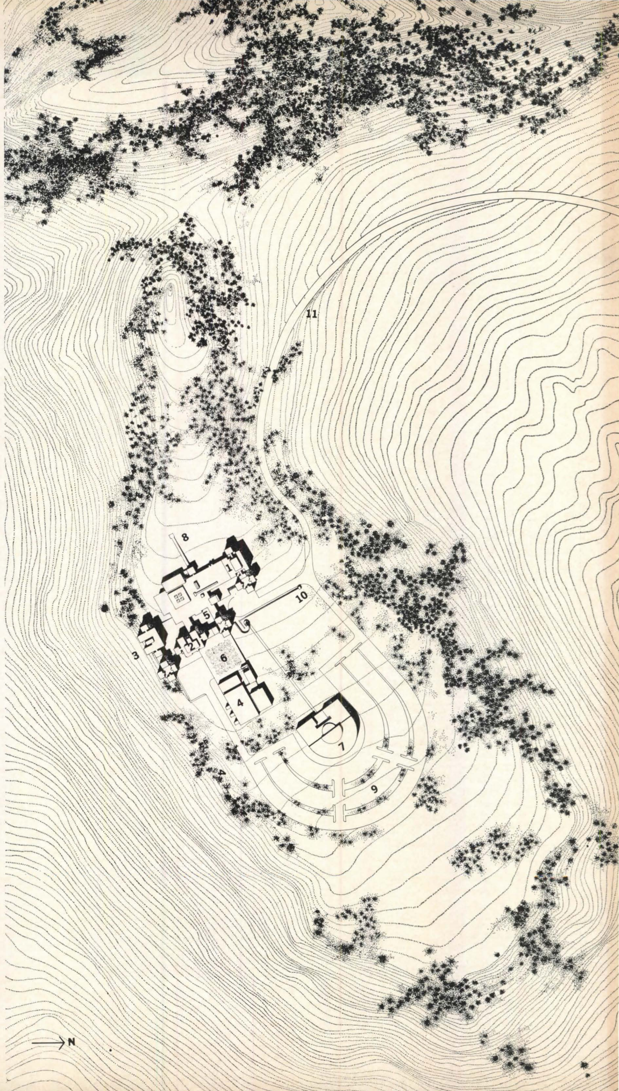
THE SITE—At left, the view of the mesa from the east. At right, the various elements of the center, both built and projected: 1. office complex; 2. laboratory complex; 3. future office and laboratory complex; 4. future laboratory; 5. enclosed plaza; 6. open plaza; 7. future conference building; 8. ramp to west mesa; 9. parking lot; 10. sculptured gatepost at main entrance; 11. approach drive to NCAR complex.
