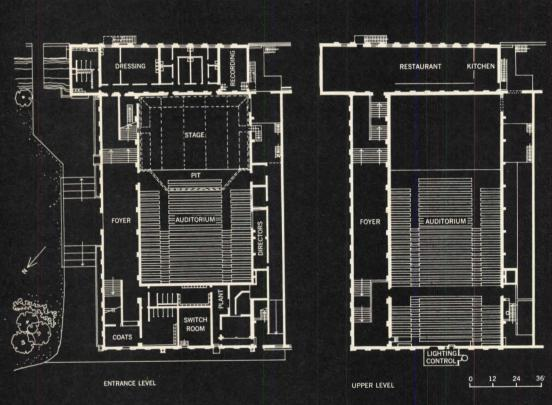
WALLS AND FLOORS: Top picture shows new terrace outside main entrance. It was paved with a local brick similar to the one used in the old buildings. Plans show two levels of the building as remodeled. Foyer, seen in view on opposite page, has original brick walls and a floor of a special local tile no longer available in the area.
