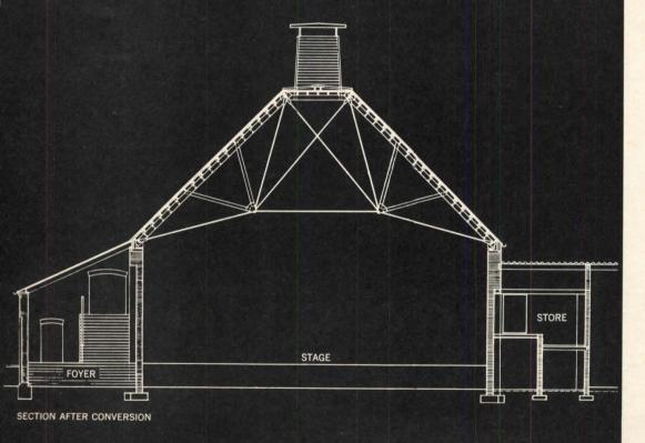
SECTIONS—BEFORE AND AFTER: Old roof was removed entirely, as was the third brick wall from the left. New roof structure rests on old walls raised 2 ft. and stiffened with arches. Pitch of new roof is 45 degrees. Four new ventilators were prefabricated to resemble the traditional smoke hoods nearby.
