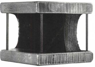
Random samples of silicone and Tested-Approved polysulfide-base sealant compared in expansion test.
