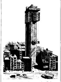
The rendering in our April issue, which did not show the proper construction sequence, was supplied by Mr. Gorsline himself. The correct sequence of assembly --from top to bottom--is shown in the revised sketch above.--ED.
