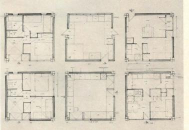
Drawings on these two pages explain the basic organization of the building: at far left are the floor plans, from the lowest floor up to the roof garden, and showing only the column-and-beam grid on each floor. At near left are some of the modular unit plans that were fitted into this grid living units, kitchen-dining-maid'sroom units, and sleeping units. These were grouped around the vertical circulation core shown in the section.
