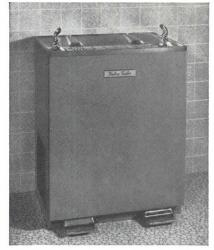
HT SERIES LOW LEVEL FOUNTAIN Thirty inches high ... especially suitable for elementary school cafeterias. Stainless steel top. Individual, self-closing, foot-operated valves with automatic stream regulators. Gray baked enamel or available in stainless steel. Dual projectors or projector and goose neck filler optional.
