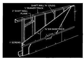
In non-bearing assembly, laminated gypsum coreboard 2" thick is installed between metal H-studs or C-channels, 24", 16", or 12" o.c. J-runners anchor panels to floor and ceiling. SHEETROCK\* SW Gypsum Wallboard is screw-attached to coreboard.
