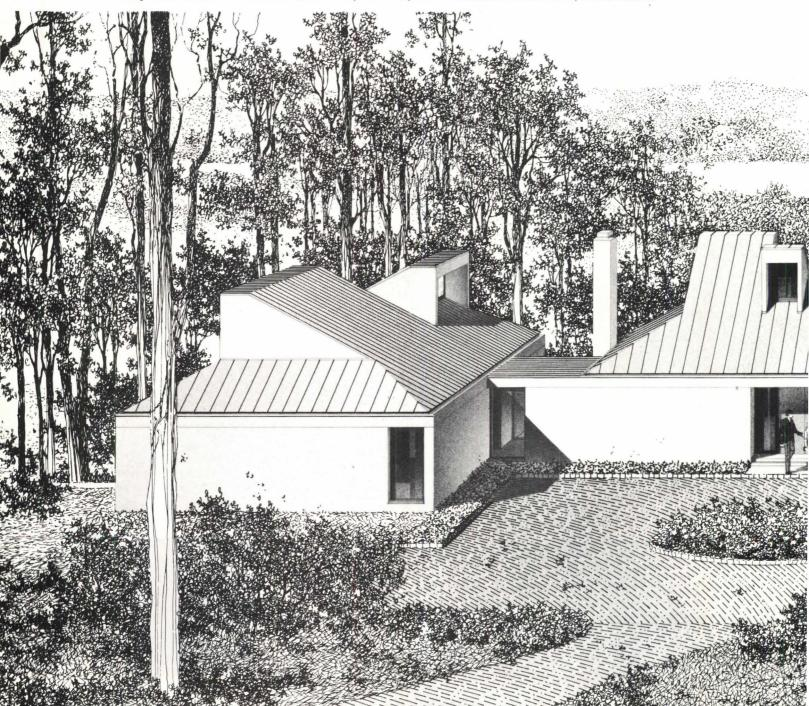
By coating 304 nickel-chrome stainless steel with Terne alloy (80% lead, 20% tin), an end product is created in which the superior qualities of both time-tested components are materially enhanced.
