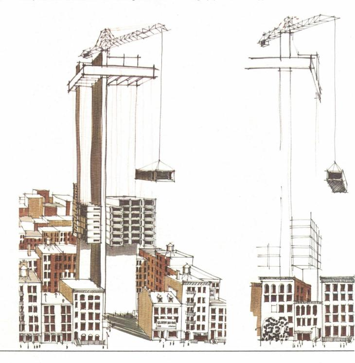
accessories, and interior and exterior finish. Deliver the completed dwelling units by truck and trailer to the building site, and put them in place around the core with a derrick on top of the core.
