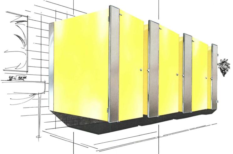
Sanymetal recesses all door hardware . . . hinge brackets do not overlap pilaster . . . hinge castings nest in precise, performed recesses providing a smooth, flush, safe and sanitary surface. Latches are internal and quiet doors ride level on concealed thrust bearings.
