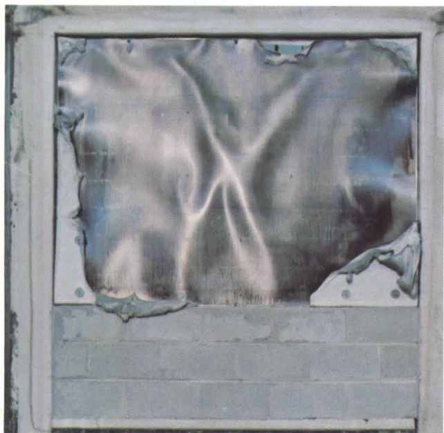
▲ Identical fire testing of glass fiber curtain wall insulation resulted in melting and general deterioration within twenty-six minutes.
