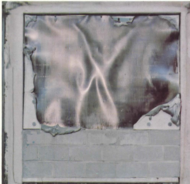
▲ Identical fire testing of glass fiber curtain wall insulation resulted in melting and general deterioration within twenty-six minutes.
