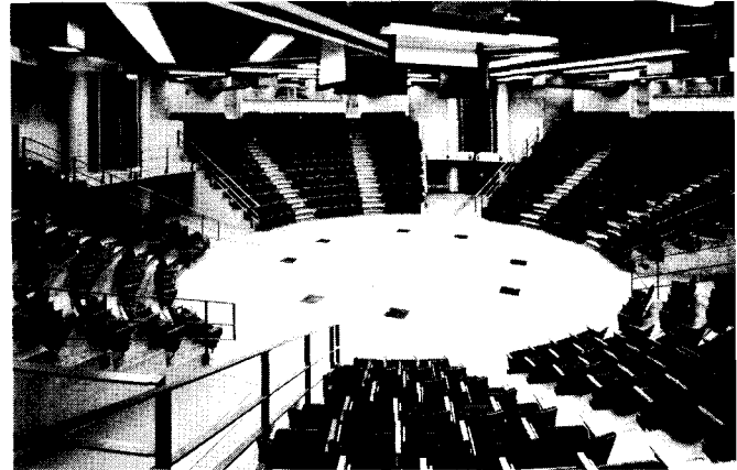
An arena stage theater (below) has been incorporated into the cylindrical wing of the megastructure. Double-coiled wood screens roll on tracks and can divide the 1000-seat theater into four quadrants for various uses. This wing, connected to the classroom building by roof and a glass-enclosed bridge, can operate as a community center at night without the rest of the building being open. Poured concrete beams, ten feet deep, span 88 feet over the auditorium in a cross-arrangement to carry the library above.
