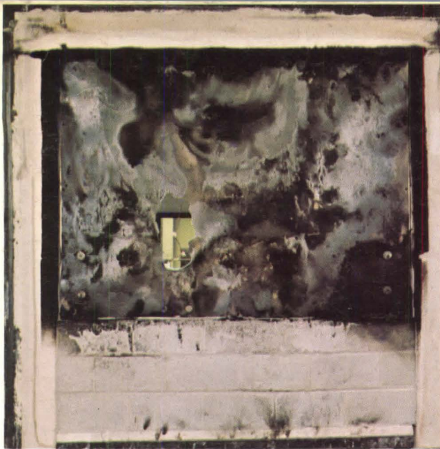
▲ Furnace fire comparison test at the U.S.G. Research Center resulted in complete disintegration of polyurethane foam insulation within five minutes.
