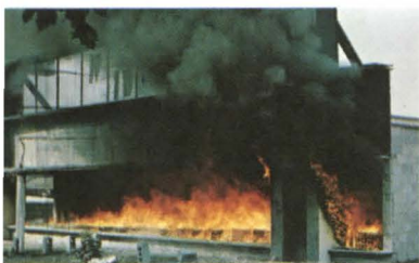
To prove that flame-shielding works, tests were conducted on a full-scale mock-up.
