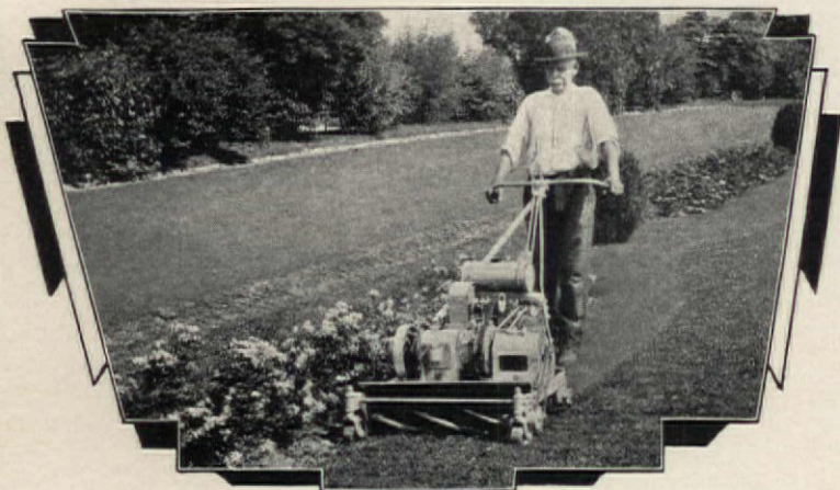
Above: Coldwell "Twin-Thirty" motor lawn mower and roller. Mows and rolls simultaneously 6 to 8 acres a day.
