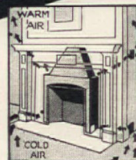
Heatilator concealed in fireplace draws cold air from floor, warms it, and returns it to the room.
