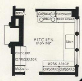
The floor plan shows the compact arrangement of equipment. The chimney projecting into the room was a decided advantage as it provided recesses—one for a tray closet and the large enough for refrigerator and broom
