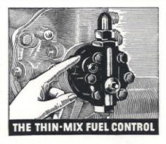
You know how a too-rich mixture in your car wastes fuel. Oil burners that lack proper controls let mixture of oil and air get too rich... waste fuel... cause smoke and soot. The Thin-Mix Fuel Control offered only on Delco Oil Burners—keeps the mixture thin... creates a clean, hot flame that gets more heat from the oil... saves money, heats your home for less cost and does it better. It's another modern miracle from the world's foremost builders of devices for combustion of liquid fuels.
