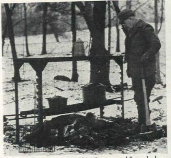
Mark A. Kindig cooking on a large "picnic grounds" stove he designed. The cooking area is adjustable, the fire being on the ground
