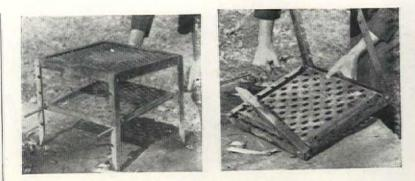
Above left: The folding stove's fire pan can be raised or lowered. Right: Folding the stove so it can be stowed in an automobile or boat
