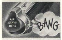
This remarkable safety tube consists of a reserve two-ply inner tire inside the regulation tube, both inflated by the same valve. When the casing blows out only the outer tube lets go. The inner tire holds enough air to support the car without lurching until you can come to a safe stop
