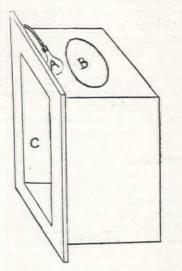
Fig. 1. Shadow box construction. A-Electric light bulb; B-Oval opening in top of box; C-Front opening to be screened with white paper
