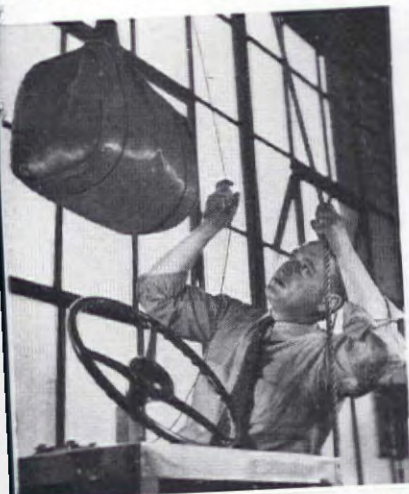
4 Rubber He Can't Break even with this 200-pound weight. Plymouth's sturdy steering wheel is made of hard rubber, with a solid steel core.
