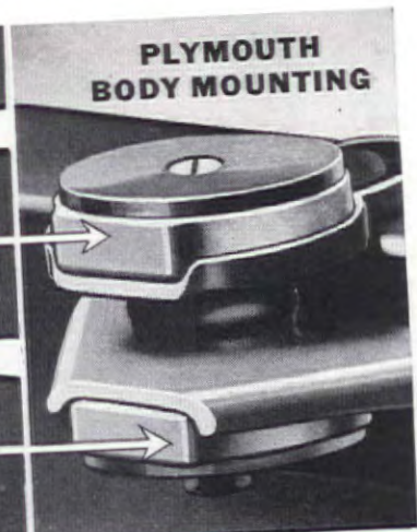
3 Your Backbone is Cushioned (left) by pads of cartilage or "gristle"—in much the same way Plymouth's body is cushioned (right) on its "live" rubber mountings! These cushions block out shocks, noise and vibration. Plymouth's famed Floating Power engine mountings work the same way.
