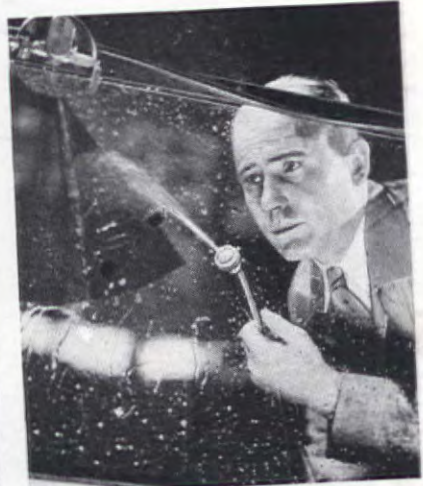
6 Wiper Tests —Not only the mechanism but the rubber is tested as in the many other parts of the car where this material means long life.
