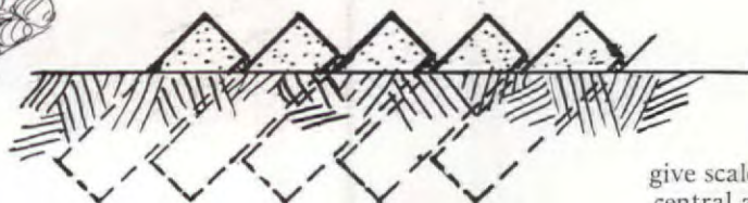
Law-tooth brick Kerb, bricks set diagonally at end, deeply bedded in earth.
