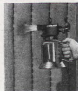
Fire-Resistant KIMSUL is non-burning. When exposed to flame, a KIMSUL blanket merely chars.
