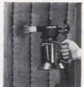
FIRE-RESISTANT —KIMSUL is non-burning. When exposed to flame, a KIMSUL blanket merely chars.
