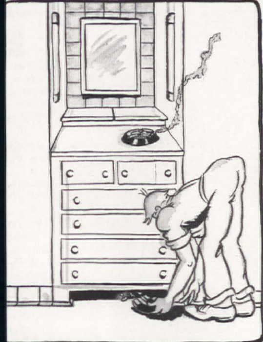
BUILT-IN, RECESSED CHEST OF DRAWERS FOR MY IMAGINARY DRESSING ROOM. THE WALL ON WHICH THE MIRROR HANGS IS OF GLASS BRICK. CHEST ALLOWS FOR TOE ROOM— IS OTHERWISE SET SOLIDLY ON THE
