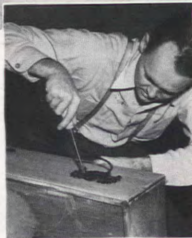
Hardware is removed before application of varnish remover
