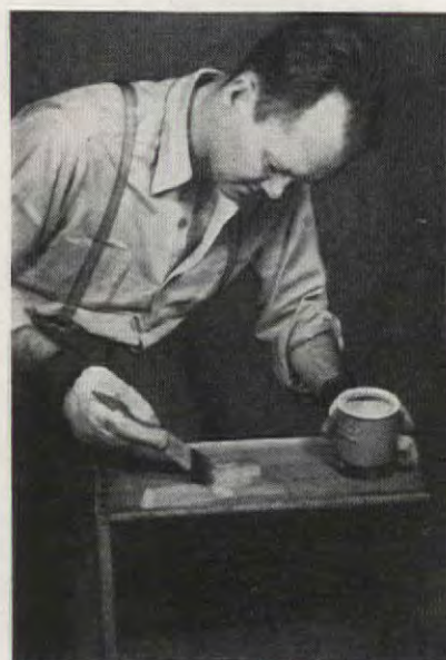
After removing dust raised by sandpaper, wood is ready for finish. To produce blond cast, brush on resinous white paint
