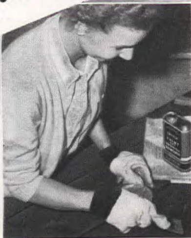
First step in refinishing process is application of varnish remover
