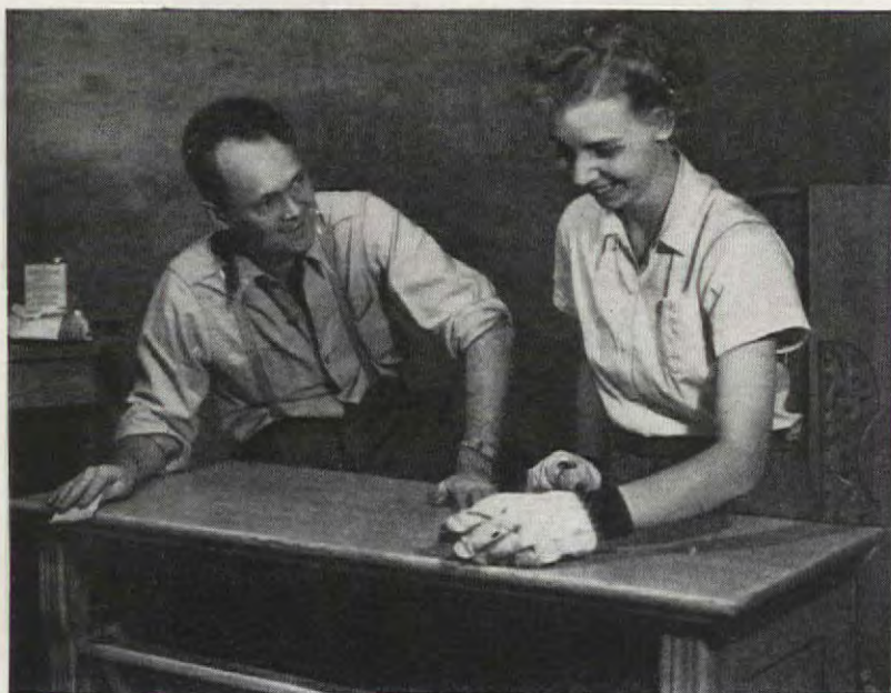
After varnish has been pretty well removed, sandpaper all surfaces first with coarse, then fine, emery paper, working with wood grain
