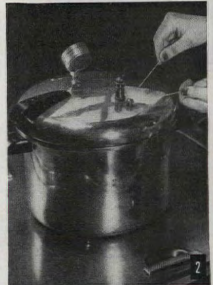
2. Clean pet cock and safety valve by drawing string or strip of narrow cloth through them
