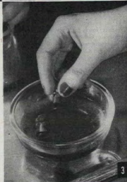
3. Occasionally remove pet cock and safety valve and soak in vinegar for a short time
