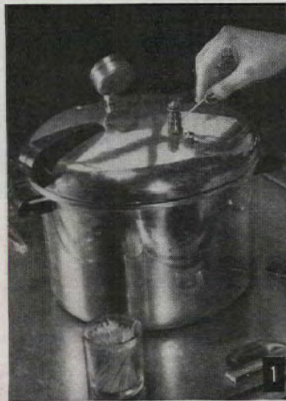
1. Clean openings to pet cock, safety valve, pressure gage, with a toothpick or another sharp tool
