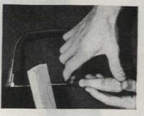
A coping saw will prove most handy when cutting the curved lines which add so much grace to this all-purpose utility table
