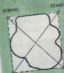
Fig. 2 To center a sprinkler head in irregular area, locate the intersection of the diagonals of the completed rectangle
