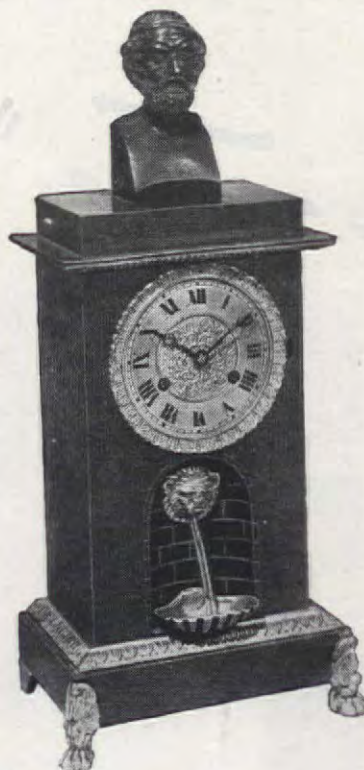
Fountain clock: spun glass spray creates illusion of water. First such mechanical clocks made about 1730. Has an eight-day French movement
