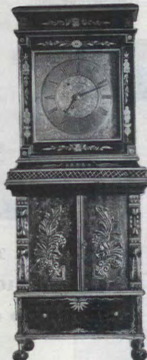
Italian Grandmother clock: movement by Carl Sormani, circa 1736, very rare crown wheel escapement numbered locking plate on back for strike
