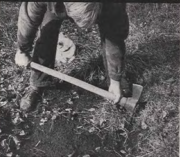
6. When digging with a mattock, don't lift or tear it forcibly from the ground after each stroke. Again use leverage. Push down with the hand at the handle end, using the other as a fulcrum; then lift with both arms. When you get the point under a rock, pry, don't pull, it out
