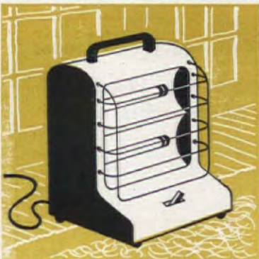
Electric outlets for heaters must provide from 1,000 to 2,000 watts, depending upon size of heater
