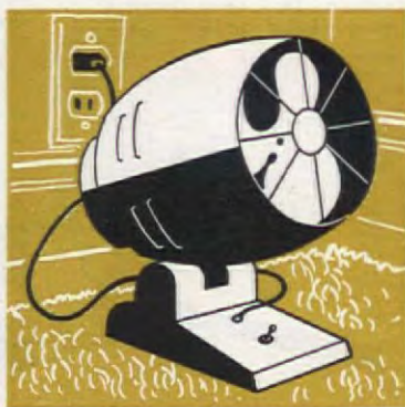
Most portable electric heaters produce heat by radiation; some combine radiation with convection
