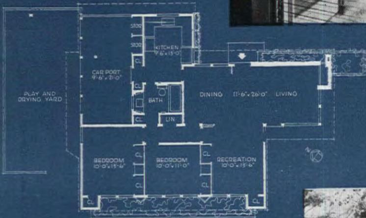
● Revere Quality House is as modern in detail as it is in plan. Opaque Ventaglass assures privacy, at the same time affording maximum ventilation through doors; car-port door slides shut to form wall extension. In plan, outside entrance from garage through kitchen to bathroom makes it ideal for children, saves muddy footmarks in main house; flexible partitions make one room out of three
