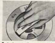
2. Lock protecting cover with a twist to the left. Notice openings in the cover for clean, flushing water to enter the Disposall as it works.
