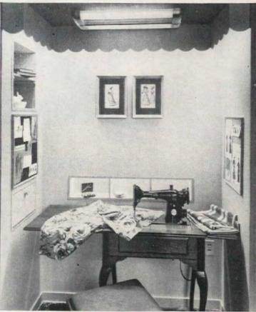
As sewing alcove, more light is required. Fixture on ceiling directs additional light onto sewing machine with minimum of shadows on work surface. Perimeter lighting furnishes general illumination
