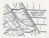
remedy small leaks. Larger holes should have the additional protection of a piece of roll roofing or asphalt roofing felt pressed into the asphalt cement and covered with another coat of the cement. Separate leaks, where a general bad condition doesn't exist, can be handled in a similar manner for a quick and easy repair during cold weather when soldering would
