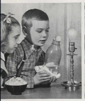
FOG in a milk bottle. All you need is a cup of hot water inside, a cube of ice on top
