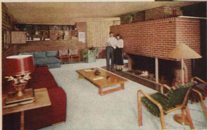
● Study, living, dining, kitchen activities are all encompassed in large rectangle with minimum divisions. Oversized fireplace in center of room has two flues, burns 10-foot logs or 2 twin fires
