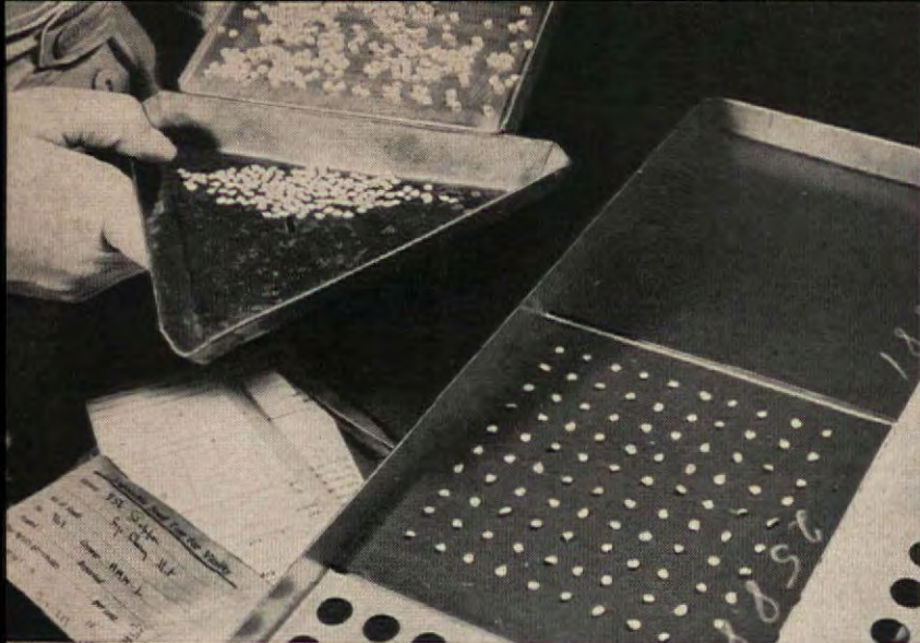
Countless samples are analyzed in many ways. Here 100 seeds are spaced, held by air suction while excess seeds are poured off
