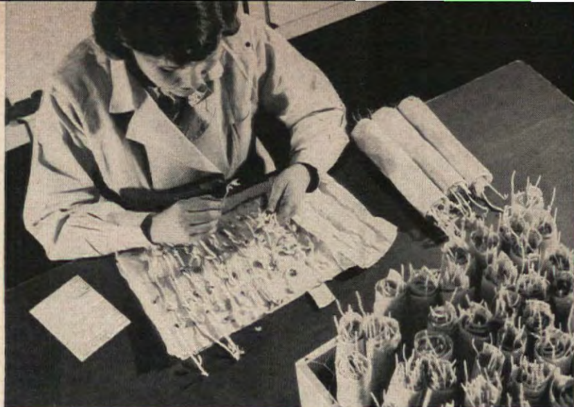
Some test lots are spread on moist paper towels, rolled, and put in heated cabinets to germinate. Here, results are counted
