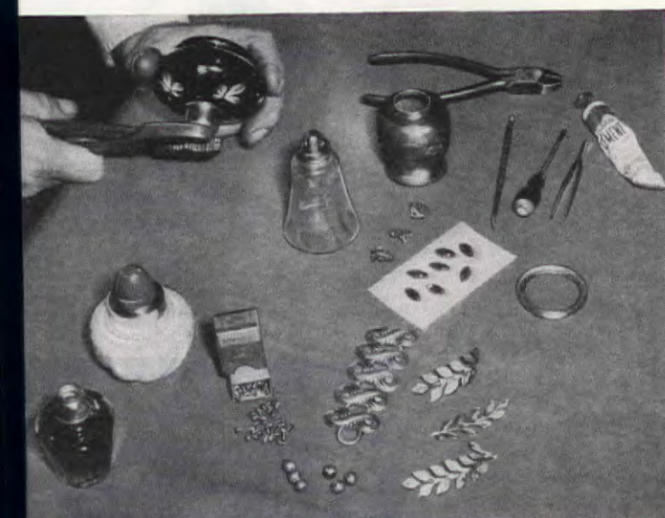
Basic materials gathered to make miniature lamps. Costume jewelry serves as base feet and decorative trim, bottles as lamp parts. Bottle necks are removed and replaced with metal necks
