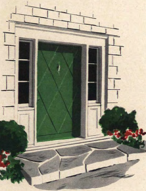
Diamond-shaped pieces of plywood, set \frac{1}{4} inch apart, were applied to face of this entrance door. Since the added plywood will make the door thicker, frame stop must be moved back to bring door flush with trim
