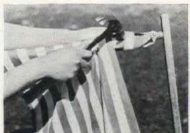
After fastening bottom end, tack top from side to middle as shown
