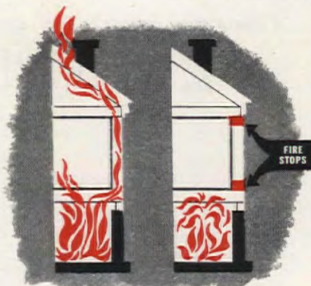
Fire stops between studs keep flames from spreading quickly in walls and enveloping house. An alarm system to warn of danger gives still more time for escape and fire-fighting
