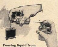
Pouring liquid from a bottle into a small hole as when filling a lighter is quite a trick without a funnel. But a wood match or a toothpick held across the bottle opening as at A will guide the liquid directly into the target without spilling and wasting the fluid when you start pouring
