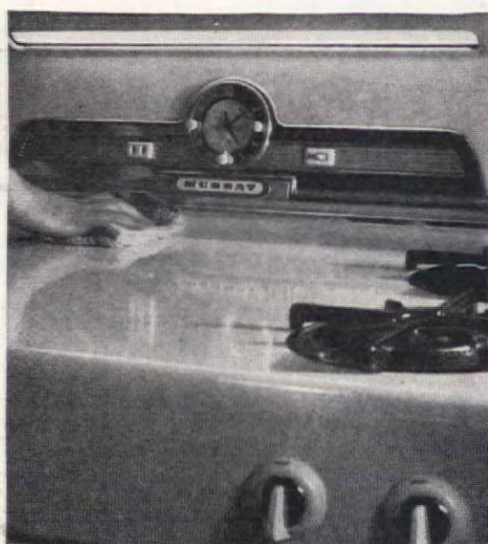
To overcome unsightly walls which come from ranges' venting at back, Murray places almost invisible vents across front of their range backplash. Grease is deposited on range top, is simple to wash off with each use
