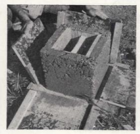
11 If box is too rough, apply rich cementsand mixture. Grasp handle and pull out inner mold, tapping it gently and carefully with hammer to free it if necessary (see 12)
