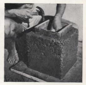
12 If drain hole (made by cork) does not go through concrete bottom, open it up with screwdriver. Use molds to make more boxes. (Suggest oiling form faces with heavy oil. Ed.)
