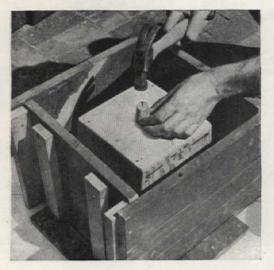
7 Nail large cork in exact center of top of inner mold to provide a drainage hole in the finished pot. It must not protrude higher than the highest part of the outer box or form
