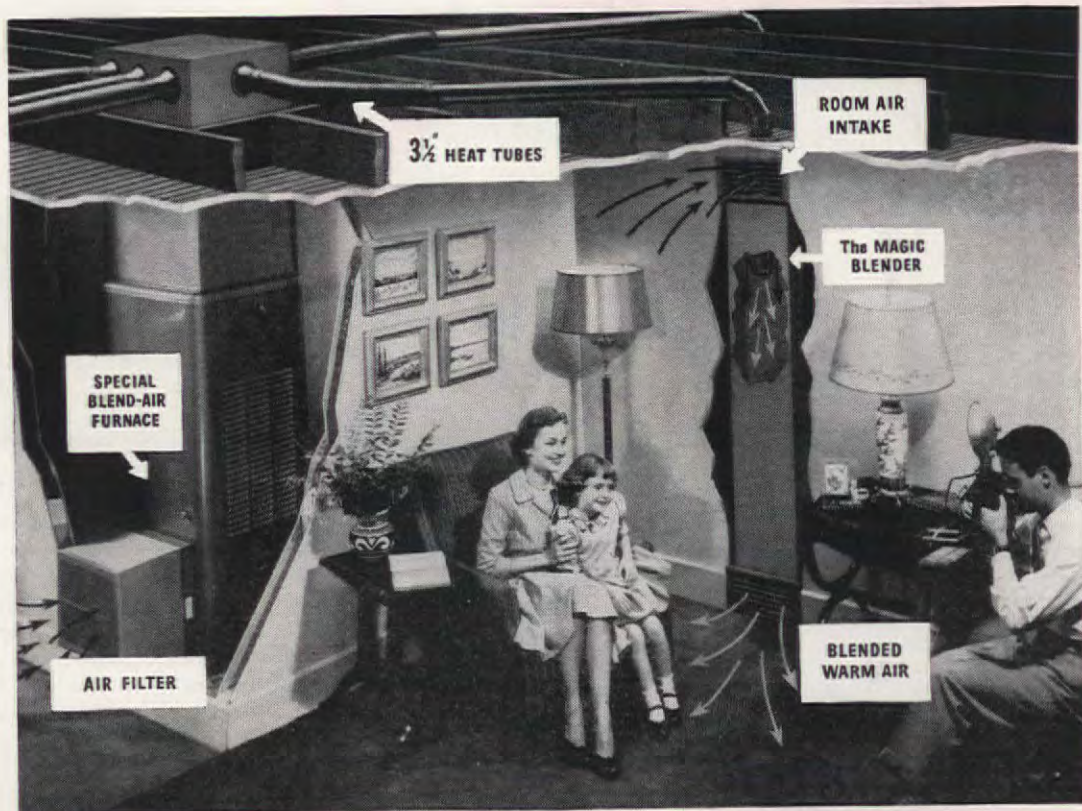
This illustration shows a Coleman BLEND-AIR installation with the furnace located in the utility room. Heat Tubes are located in the attic. In basement installations, the Heat Tubes are located in the basement immediately beneath the floor.
