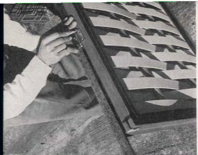
14. Two hinges were used on this screen. Square two completed framed panels. Measure down 14 inches from each end, lay hinge on frames and mark a guide line. Hold firmly in place, screw tight
